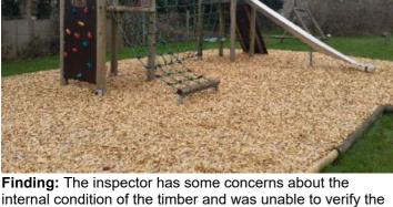
Finding: The inspector has some concerns about the internal condition of the timber and was unable to verify the structural integrity without further testing. We recommend a Resi-PD survey to establish the condition of the timber at it's core.
